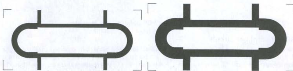
Fig. 5 PCB patterns of the hybrid power combiner – not to scale
